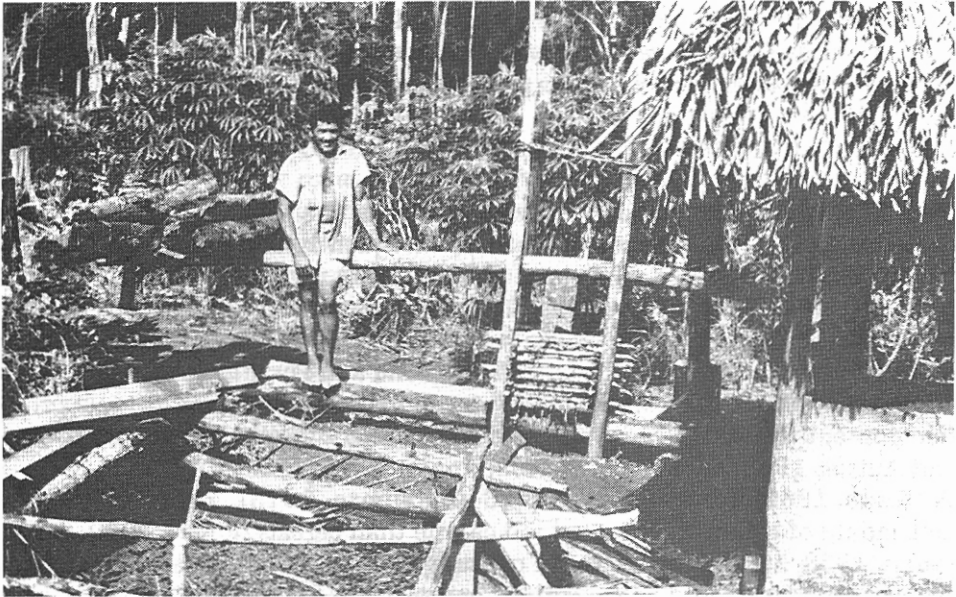
Fig. 2. One of the several kinds of manioc press used along the Transamazon. Note the casa da farinha on the right. Km 400 Altamira-Itaituba, October 1973.
